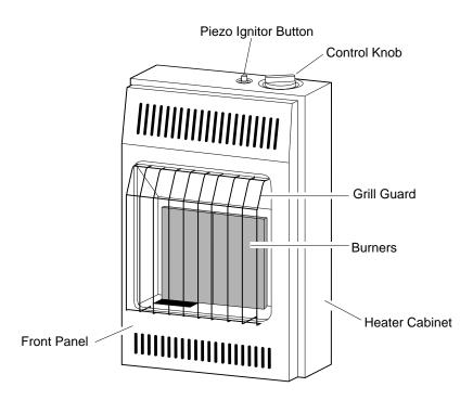
Figure 1 - Model VN10TA Vent-Free Natural Gas Heater
